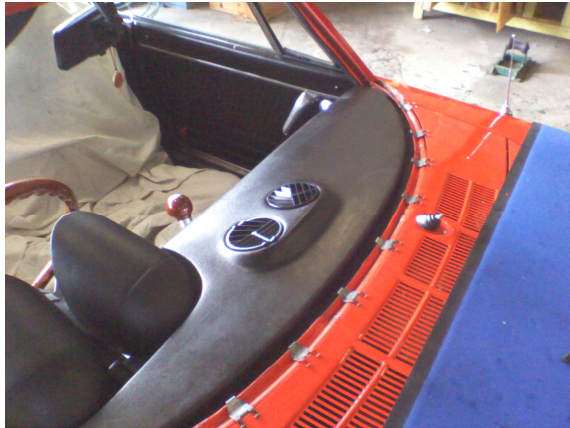
Above: Windscreen frame cleaned and ready for the new glass. The bottom clips hold the stainless-steel trim in place
