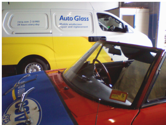
Above: Car prepped and stainless steel windscreen trim removed.
