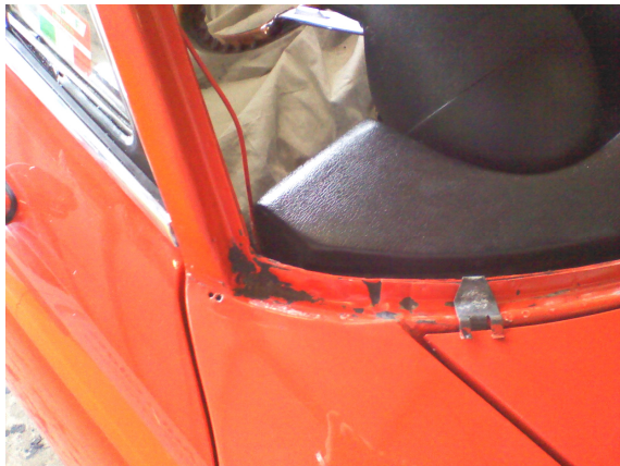
Above: Close-up of driver's side bottom corner, showing original paint and scars from a previous windscreen replacement
